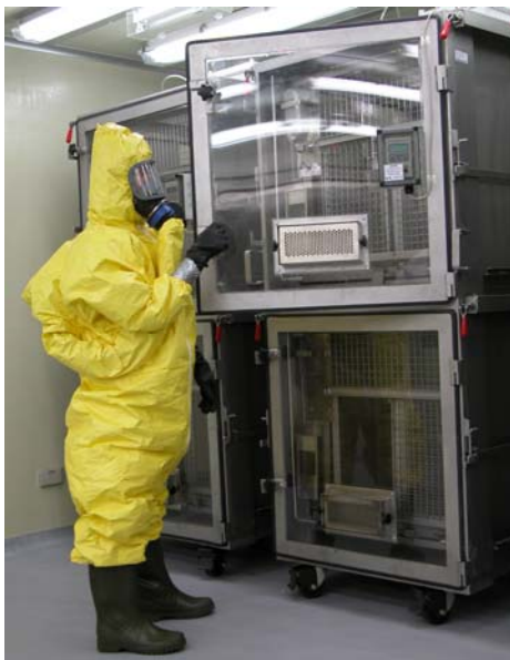
Fig. 1. The BSL-3 facilities and building established in Animal Health Research Institute. The BSL-3 lab was established in the National Animal Diagnostic building. The BSL-3 lab contains negative pressure system and human protection facilities.
